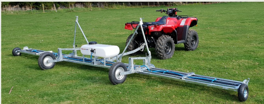
Wipe Out 6.2: 6.2m wiping width
